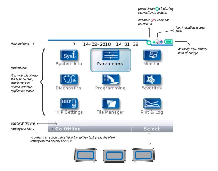
In this above example, pressing the "Select" softkey will open the highlighted Parameter app. The "Select" softkey opens whichever app is highlighted. Pressing the "Offline" softkey switches the 1313 HHP to Offline mode. In Offline Mode, the 1313 HHP cannot communicate with the controller. The 1313 HHP can perform operations that do not require communication with the controller. See Chapter 15.
