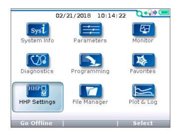
The **HHP Settings** app allows adjustment to the appearance of the screen displays and the 1313 HHP's functionality. Highlight the "HHP Settings" icon and press the "Select" softkey to enter the app. The app is accessible when working offline. Return to the main screen at any time by pressing the main screen key (...).
