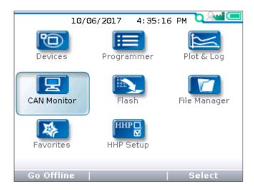
In the main screen, highlight the CAN Monitor icon and press the "Select" softkey to open the app. Return to the main screen at any time by pressing the main screen key ( ).
