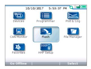
Use the Flash app to obtain and save parameter values, restore (load) parameter values to the device, or update the device's firmware. Highlight the Flash icon and press the "Select" softkey to open the app.
