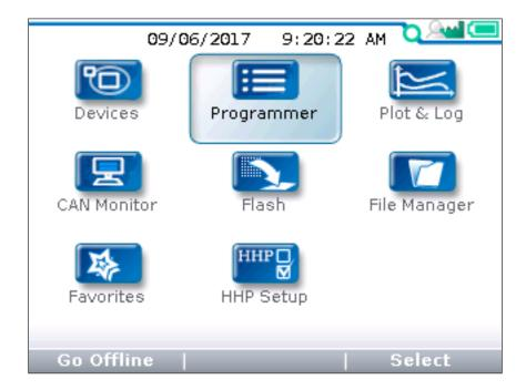
To select an app, scroll using the arrow keys ( $\P$ ) until the app is highlighted. Apps can also be selected by successive presses of the main screen key ( $\blacksquare$ ). Each press will highlight the next app.
