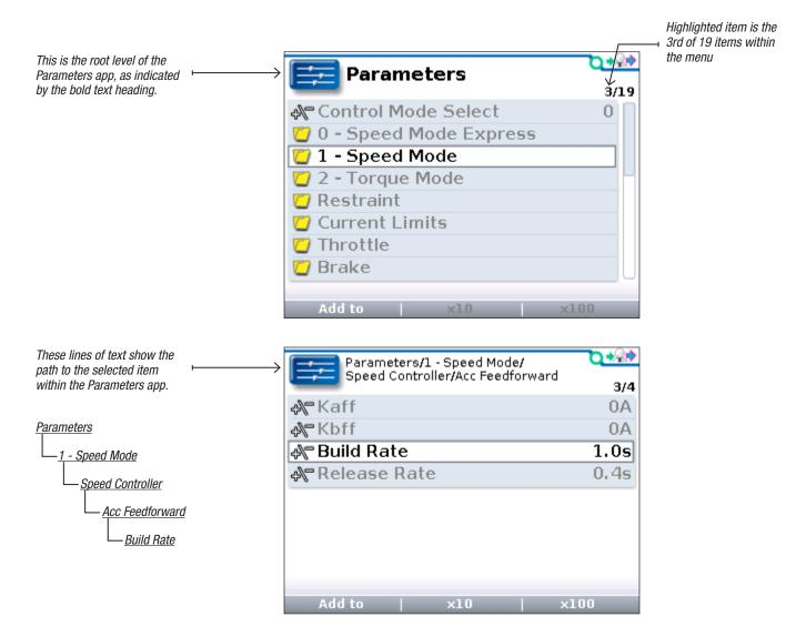
Note that when the Speed Mode folder is highlighted, the "×10" and "×100" softkeys are grayed out (indicating they do not apply)—but when Build Rate is highlighted, these softkeys are available.
