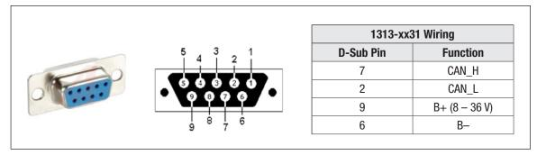
Vehicle Harness Wiring for CAN Connected 1313 HHP
