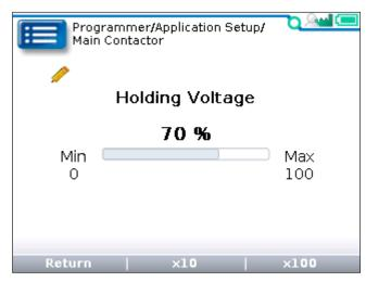
Holding Voltage expanded (detail screen example)
