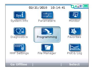
Use the Programming app to obtain and save the parameter values, or restore (download) parameter values to the controller. The parameter settings are saved in a dedicated Curtis Program File (.cpf) format. A .cpf file can also be opened and viewed using the 1313 HHP offline mode (see Chapter 15). In the main screen, highlight the Programming icon and press the "Select" softkey to open the app. Return to the main screen at any time by pressing the main screen key (...).
