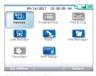
(2) Main Screen following the CANbus scan Just the "Offline" capable apps are available.
