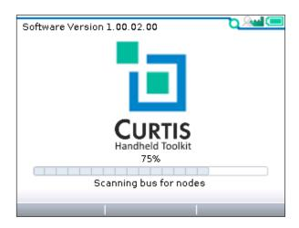
(1) 1313 HHP startup-scan of CANbus for devices
