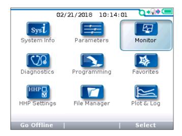
In the main screen, highlight the Monitor icon and press the "Select" softkey to open the app. Use the arrow keys and the softkeys to navigate within Monitor. The Monitor menu provides real-time data of the monitor variables. It is recommended that the controller manual be consulted for explanations of the monitor variables.
