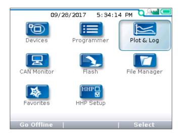
In the main screen, highlight the Plot & Log icon and press the "Select" softkey to open the app. The Plot & Log app has a Plot utility and a Log utility. The Plot utility plots the values of selected variables over time. The Log utility creates a log with the values of selected variables over time. The log can then be viewed in a spreadsheet program on a PC. Return to the main screen at any time by pressing the main screen key (...).
